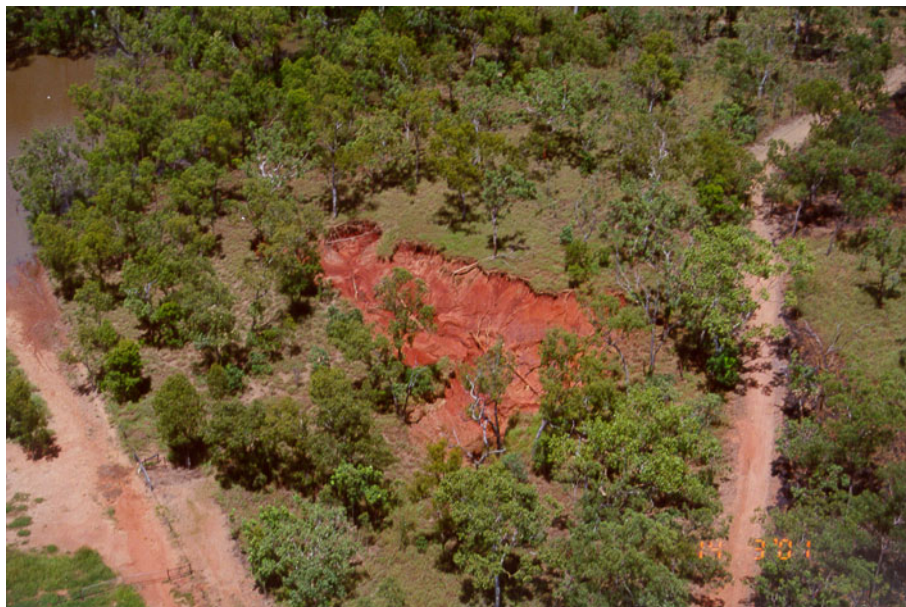
Plate 10 Example of suffosion sinkhole formed in Cutta Cutta Nature Park (AMG co-ordinate 53L 227250-8385500)
